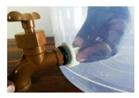
Make sure one washer is on the outside of the bucket/water storage vessel and the other is on the inside of the bucket/water storage vessel along with the backing nut screwing it firmly onto the plastic tap and against this inside washer.
